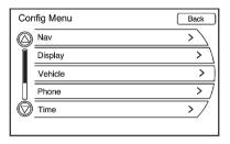
Turn the MENU/SELECT knob to scroll through the available setup features. Once the desired feature displays, press the MENU/SELECT knob or press the desired feature on the screen, to display more options within that feature
